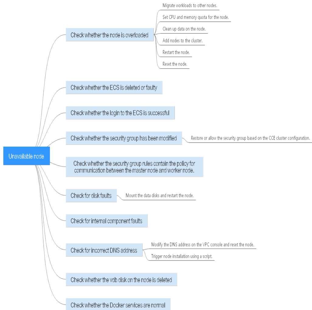
Figure 20-2 Troubleshooting process for an unavailable node
